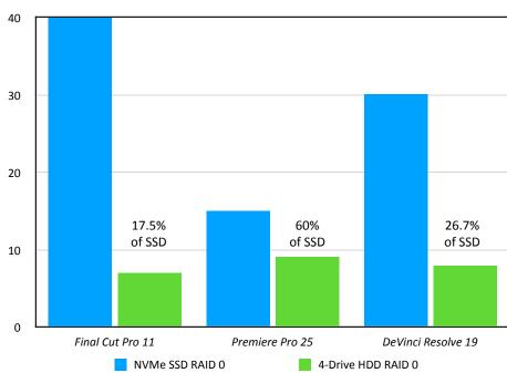
The big multicam limitation of spinning media is latency, the time it takes to move the drive heads between files.
